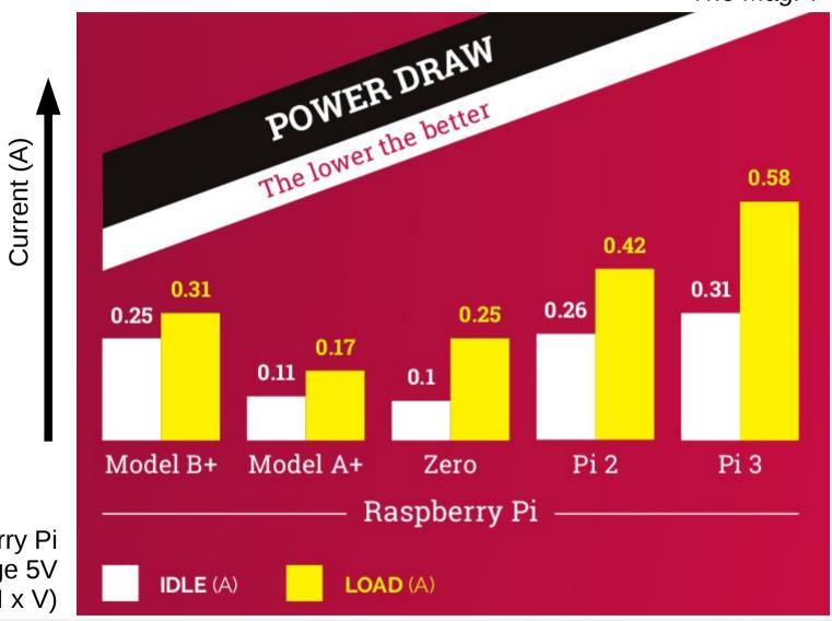
Raspberry Pi Input voltage 5V  $(P = I \times V)$
